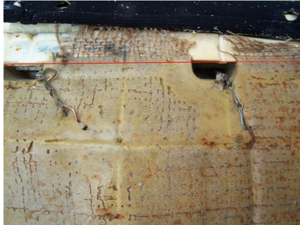
Figure 3 cut line for bolster removal
